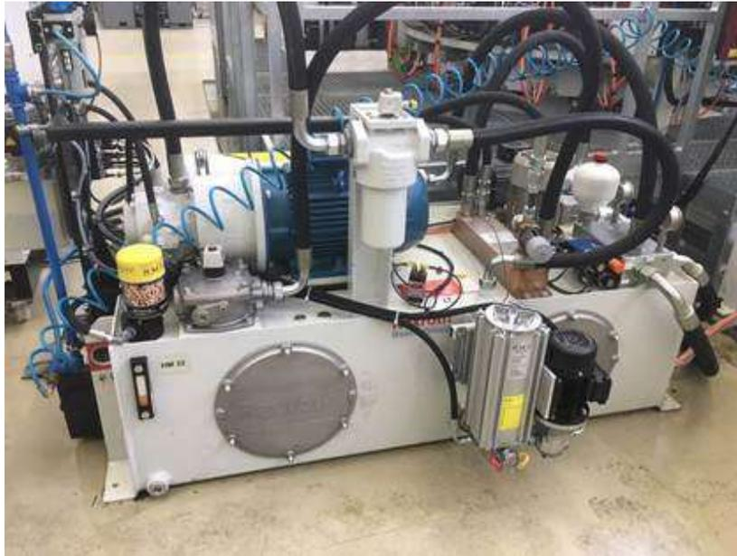
And also, examples of Hydraulic Systems modified with Des-Case Adapter Kits, to enable oil top-ups, level indication, taking oil samples, and drain oil.
