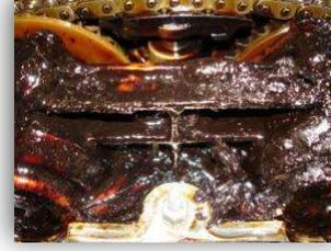
Varnish reduces clearance zones, which means a transition from hydrodynamic lubrication to boundary lubrication which increases wear rates of pumps, bearings and gears. Varnish increases friction in components which will result in higher energy requirements. Varnish acts as an insulator, lowering the effect of heat exchangers and lessening the ability of oil to cool. Varnish accelerates wear by attracting dirt and solid particles.
