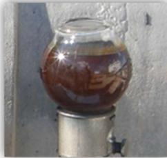
Oil quickly becomes saturated and suspended sludge makes oil appear dark and cloudy.
