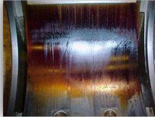
Oil comes in contact with cool surfaces and causes suspended and dissolved sludge to adhere to machine surfaces.
