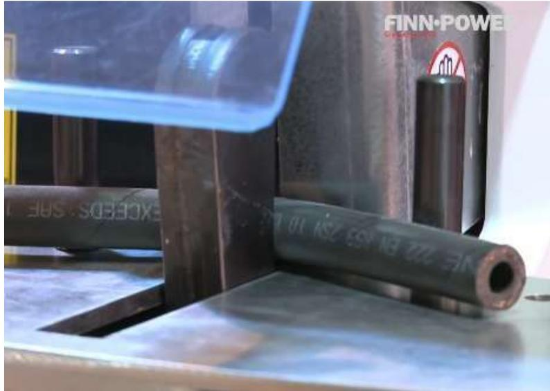
Correct equipment use for hose crimping is extremely important. Finn-power from Finland has many years of experience to create a reliable crimp.
