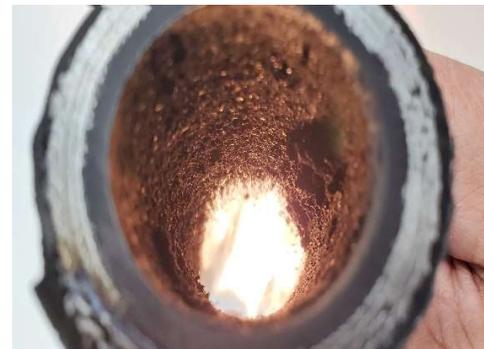
The picture here shows how the hose is unclean from inside after cutting.
