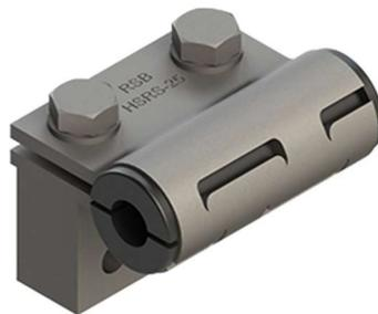
6. Sensor clamps - Fixing clamp for proximity switch according to EN 50025 and 50037. Metal parts of the standard program of series A according to DIN 3105 must be used. The sensors can be adjusted axially and laterally when mounted on mounting rails.
